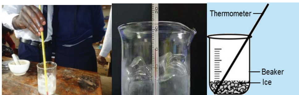
Figure 5.4: Determining the lower fixed point on a thermometer
